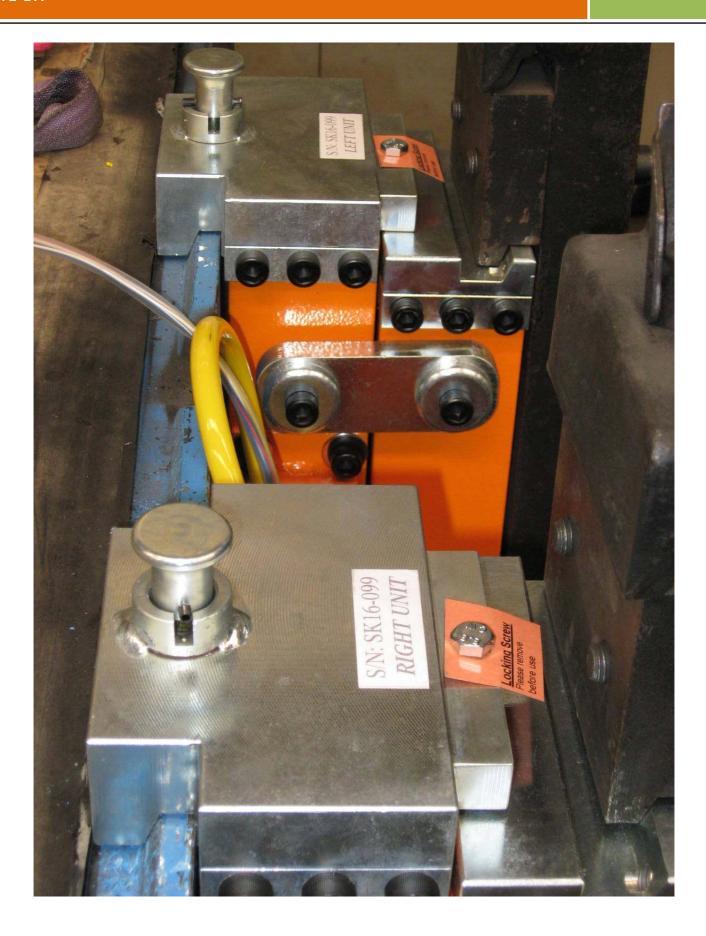
• Remove the Locking/Safety Screws
