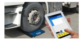
In the example, an application with wireless pad, WWSDUAL option, analogue pad, Bluetooth BLTH and DINI SMART AXLE weighing App.
