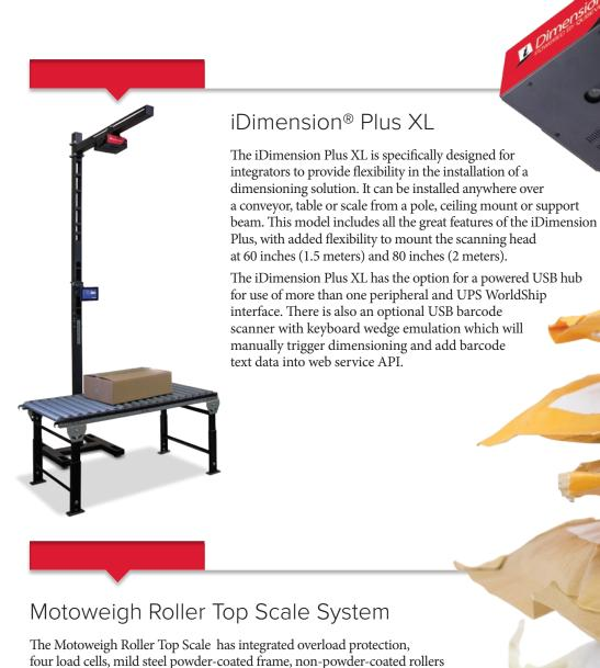
and 100 x 0.05 pound capacity and resolution. With the flexibility of the iDimension Plus XL, you can pair together to help improve the process of your existing workflow. Dimension and weigh each package in less than 1 second.
